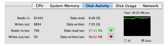
The fastest we can copy to an eSATA 2-drive RAID is about 100 MB/second.
