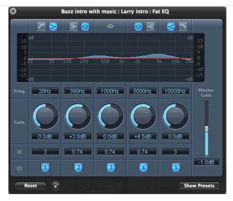
To warm up the low-end of a voice, I'll add +3 dB of gain around 390 cycles. Then, to improve clarity, I'll add +4.5 dB of gain around 5500 cycles.
