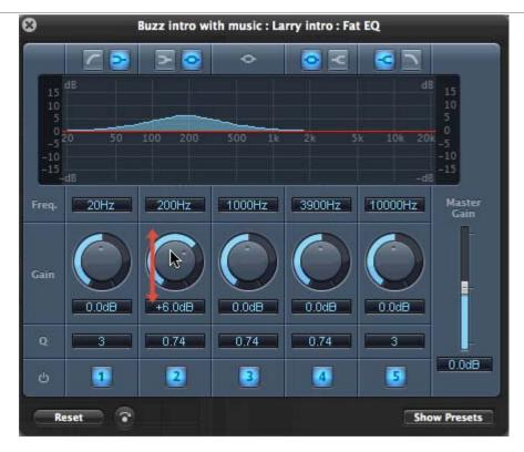
The Fat EQ filter allows us to increase or decrease specific ranges of frequencies. This allows us to change portions of the sound without changing all of it. This is very similar to color correction, where we can change the color of the shadows while not changing the color of highlights.
