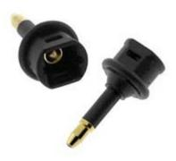
The Microphone In and Headset Out ports of ALL Macs support BOTH optical and copper signals (digital and analog). If you plug in standard audio plugs, the ports become analog. However, there's a special TOSlink adapter that turns a standard 1/8-inch miniplug into a hollow tube that light shines through. Plug this into ANY Mac and the port switches from analog to digital.
