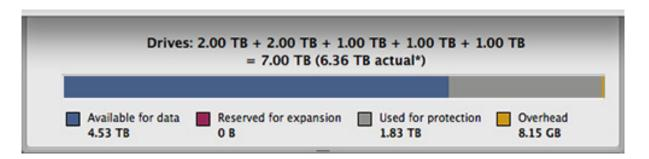
Here's how the drive space was allocated, once formatting was complete. Note that although I installed 7 TB of storage, only 4.53 TB was available. This is normal for RAIDs and I talk about it later in this issue - <u>click here</u>.
