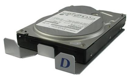
All drives were on sleds, which meant they easily slid into the unit. Assembling everything was a matter of minutes.
