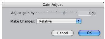
3. Go to **Modify > Levels** and enter the amount of level change into the data entry box (a negative number lowers the level, a positive number raises it)
